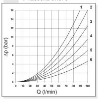
The diagram at the side show the pressure drop curves for spools during normal usage. The fluid used is a mineral oil with a viscosity of 46 mm²/s at  $40^{\circ}$ C; the tests have been carried out at a fluid temperature of  $40^{\circ}$ C.
