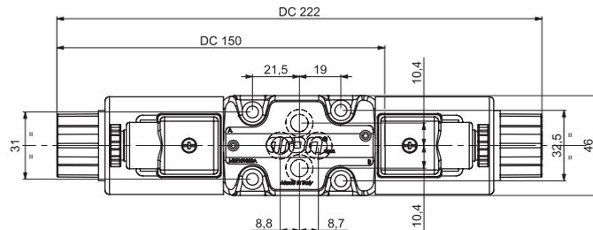
Fixing screws UNI 5931 M5x30
