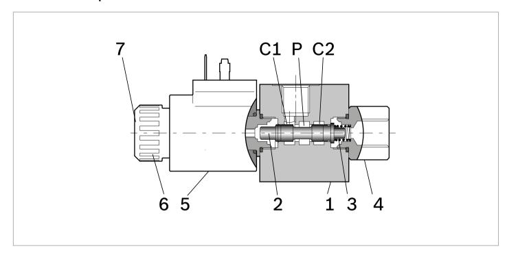
A valve basically consists of a housing (1), a control spool (2), a return spring (3) and a solenoid (5). It is designed to select which one of two circuits (C1 or C2) is to be supplied with the oil delivered from one single hose (P): with spool in position "0", when the solenoid is de-energized, the flow goes from P to C1, with spool in position "1", when the solenoid is energized the flow goes from P to C2. With the coil de-energized, the return spring (3) pushes back
