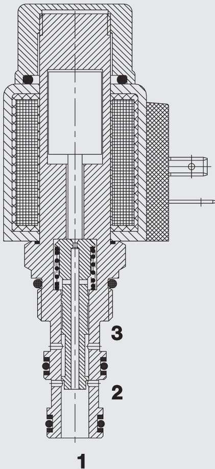
When de-energized, the valve allows flow from port 1 to 2 or from port 2 to 1, while blocking flow at port 3.
