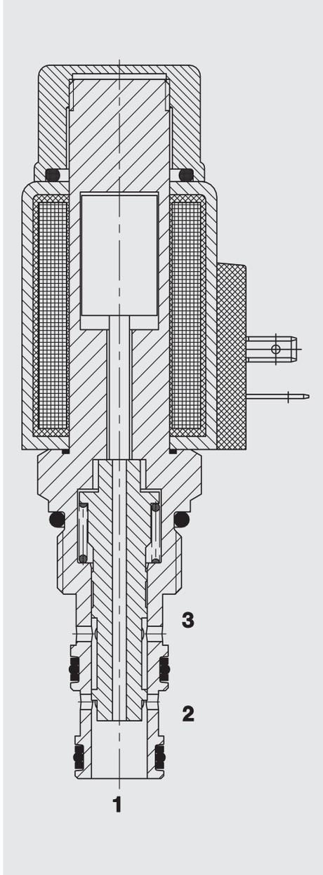
When the solenoid coil is de-energized, the valve allows flow in both directions between ports 2 and 1, while blocking flow at port 3.
