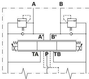
= **M0** (Relief valve with anticavitation option)
