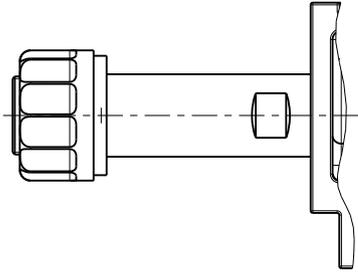
**01** Protection class: IP 65 when connector with seal is properly screwed down.
