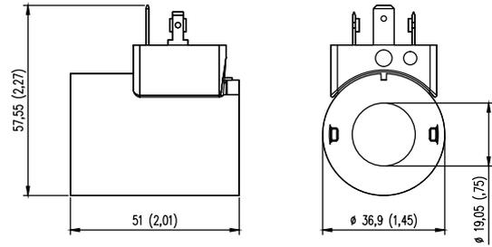
**03** Protection class: IP 67 with female connector properly fitted (see drawing).
