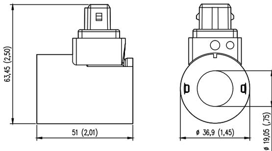
**07** Protection class: IP 69K with female connector properly fitted (see drawing).
