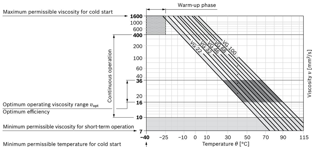
1) The FKM shaft seal is permissible for temperatures of -25 °C to +115 °C, please contact us for temperatures below -25 °C.
