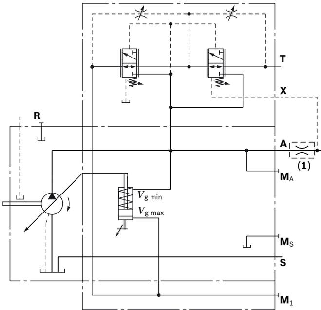
The metering orifice (control block) (1) is not included in the scope of delivery.
