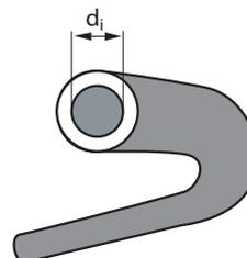
If the suction line is more than 2 m long the internal diameter must be increased by 10 mm for each meter extension.
