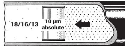
Max 64,000 particles > 5 µm/100 ml.
