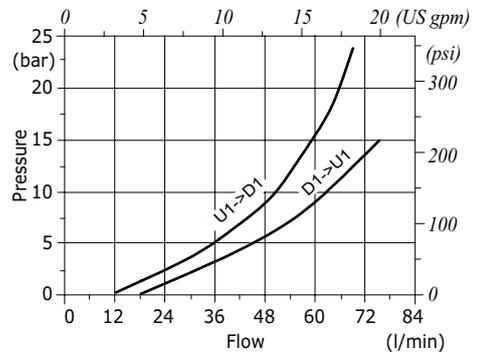
**VODL/SC 34 pressure drop vs. flow from D1->U1 and U1->D1**
